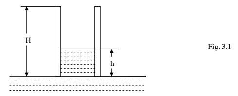
It is known: the initial intensity of the electric field of the charged capacitor, E, the density  $\rho$ , the relative electric permittivity  $\epsilon_r$  of the liquid, and the height H of the plates of the capacitor. Discussion.
