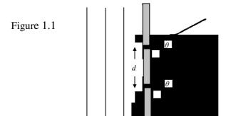
A plane monochromatic light wave, wavelength  $\lambda$  and frequency f, is incident normally on two identical narrow slits, separated by a distance d, as indicated in Figure 1.1. The light wave emerging at each slit is given, at a distance x in a direction  $\theta$  at time t, by
