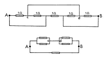
The equivalent drawing of the circuit shows that the resistance between point c and point A is  $0.5\Omega$ , and the same between point d and point B. The resistance between points A and B thus consists of two connections in parallel: the direct  $1\Omega$  connection and a connection consisting of two  $0.5\Omega$  resistances in series, in other words two parallel  $1\Omega$  connections. This yields
