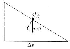
Adding up, we find that along the whole path the total work done by friction forces i  $\mu$  mg s. By energy conservation this must equal the decrease mg h in potential energy of the skier. Hence
