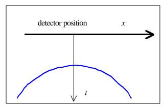
Graph of traveltime t vs detector position x,  $t_{min} = 100$  ns.
