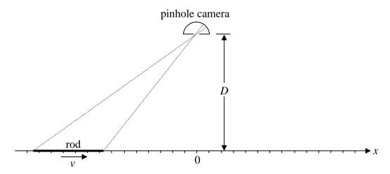
**Physical situation** A pinhole camera, with the pinhole at x = 0 and at distance D from the x axis, takes pictures of a rod, by opening the pinhole for a very short time. There are equidistant marks along the x axis by which the *apparent length* of the rod, as it is seen on the picture, can be determined from the pictures taken by the pinhole camera. On a picture of the rod *at rest*, its length is L. However, the rod is *not* at rest, but is moving with constant velocity v along the x axis.
